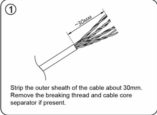
Strip the outer sheath of the cable about 30mm. Remove the breaking thread and cable core separator if present.
