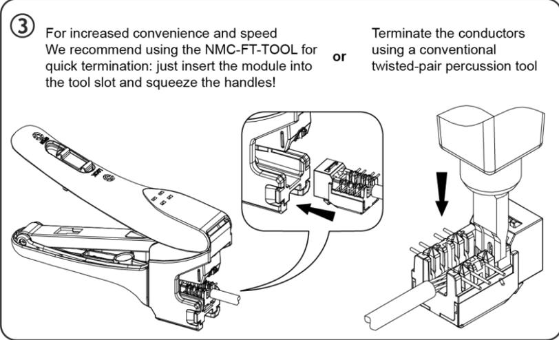
For increased convenience and speed We recommend using the NMC-FT-TOOL for quick termination: just insert the module into the tool slot and squeeze the handles! or Terminate the conductors using a conventional twisted-pair percussion tool
