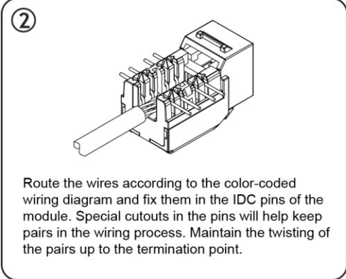
Route the wires according to the color-coded wiring diagram and fix them in the IDC pins of the module. Special cutouts in the pins will help keep pairs in the wiring process. Maintain the twisting of the pairs up to the termination point.
